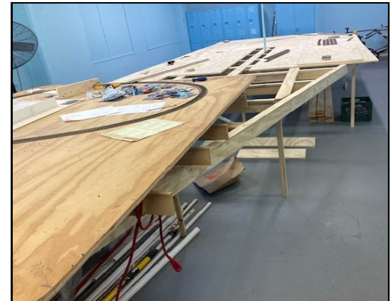
The benchwork is all cabinet grade lumber and is built to last, which is an important consideration for a layout intended for public display.
