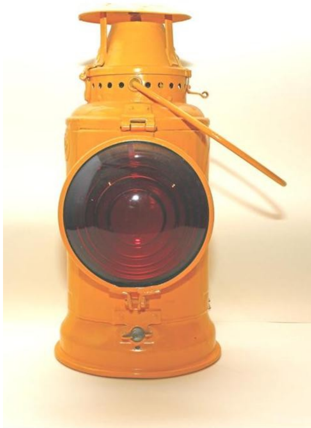
A standard Pennsylvania Railroad end of train kerosene marker lantern. These were used in pairs at end of passenger cars without electric marker lights and on the tail end of a caboose.
